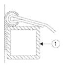
"C"TRACK ATTACHED TO HEAD BAR. VINYL EXTRUSION SEWN IN HEM SLIDES INTO "C" TRACK.
